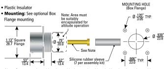
· Note: Contacts to be soldered to cable, inserted and bonded into insulator. Assembly instructions can be found at www.teledynereynolds.com or by contacting Teledyne Reynolds' Engineering.
