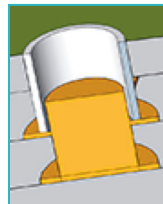
Figure 10: Insufficient back-drilling depth leaving a stub antenna
