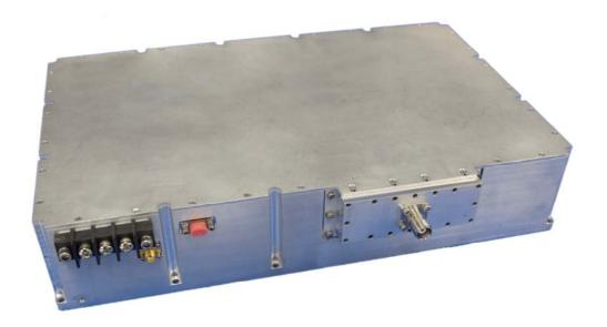
Teledyne Microwave Solutions' **350W to 1kW X-Band Solid State Power Amplifier (SSPA)** offers superior RF performance for the 9-10 GHz radar market. Designed in a compact, environmentally sealed housing, the SSPA can reliably handle any airborne or ground-based environment.
