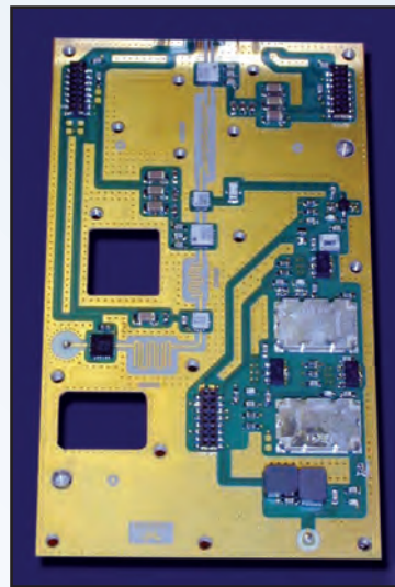
Ka-band low noise block-converter (LNB) with a typical noise figure of 1.4 dB
