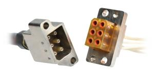
A smaller, multi-pin version of the PeeWee series of high voltage connectors and cable assemblies. Although micro-miniature in size, this series of cable assemblies will operate at voltages up to 6 kVDC at 70,000 ft (21.34 km) altitude over a temperature range of -55° to 125° C.
