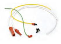
performance. In an effort to further reduce corona discharges, the SID cable assembly is available with a semi-conductive silicone wire and proprietary semi-conductive coating over the silicone plug. This configuration could also potentially alleviate the need for shielding in certain applications. The SID is rated for operation at 15 kVDC at 70,000 ft (21.34 km) over a temperature range of -55° to 95° C.
