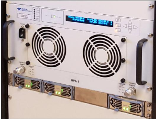
**Teledyne Paradise Datacom** manufactures a wide array of rack mountable Solid State Power Amplifiers (SSPAs) in output power levels ranging from 20 Watts to 2 kilowatts. Many of these SSPAs use an external 1RU power supply, which adds redundancy to the input power to the amplifier.
