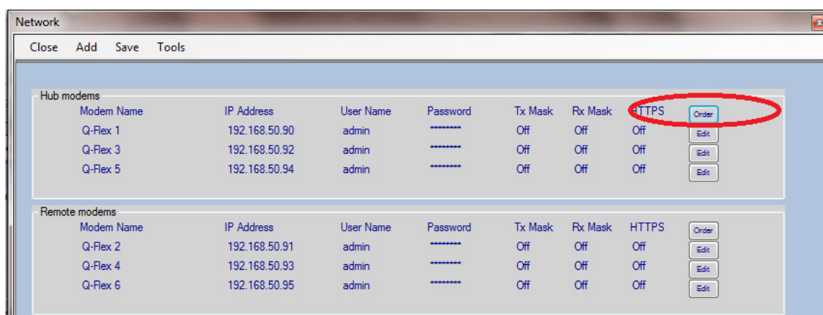
Figure 3-40 Changing the Order of Network Devices
