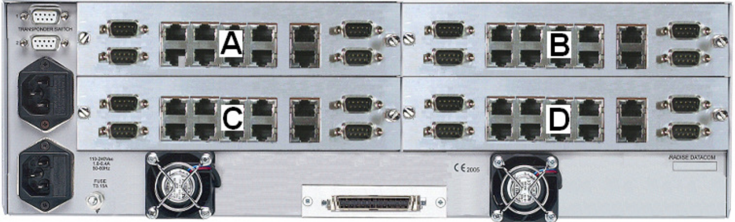
Rear view of PDQS 1:N Redundancy Switch
