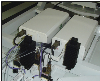
SNG-mount 1:1 system w/ side-mount AC input
