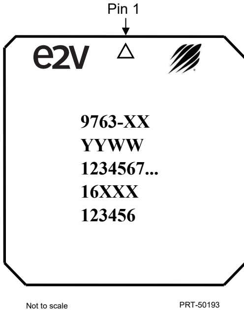
Figure 9. Top Marking Specifications
