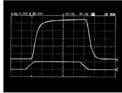
Switching speed @ 0.2 GHz, +6 dBm
