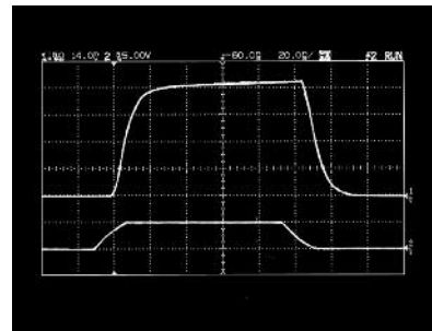
Switching speed @ 0.2 GHz, +12 dBm
