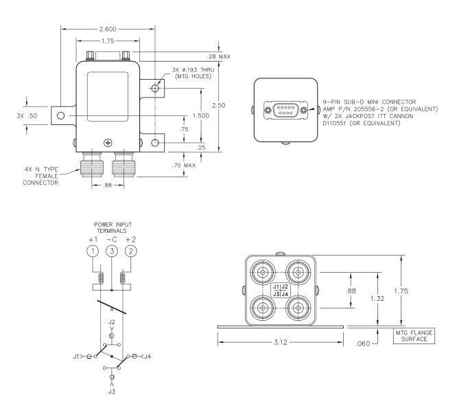
"-S OPTION" 9-PIN D-SUB CONNECTOR (EXAMPLE: CCP-47N60-S)
