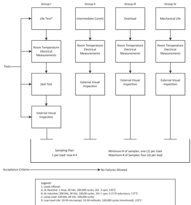
2.Intermediate Current: 100 mA, 28 Vdc, 50,000 cycles,  $10\pm1$  cpm, , 125°C
