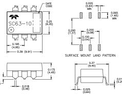
Weight: 0.035 oz. (1g) maximum Case: 6-pin dual in-line filled epoxy
