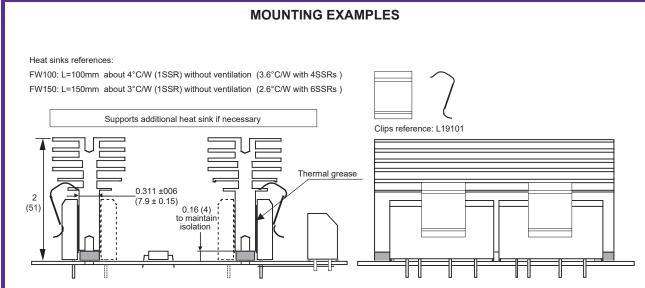
Figure 7a — Thermal heat sinks with mounting clips; dimensions in inches (mm)
