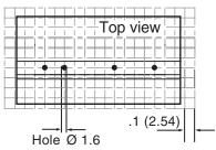
Figure 5 — LS60D22C-HS1 relay dimensions in inches (mm)
