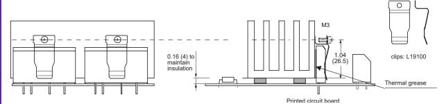
Figure 7b — Clips with screws on standard heat sinks; dimensions in inches (mm)
