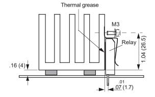
Figure 10b – Mounting with L19100 clip; dimensions in inches (mm)
