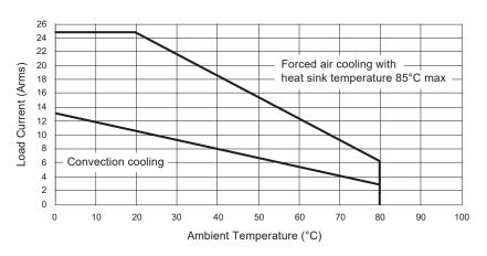
Figure 6 — LS60D22C-HS1 relay
