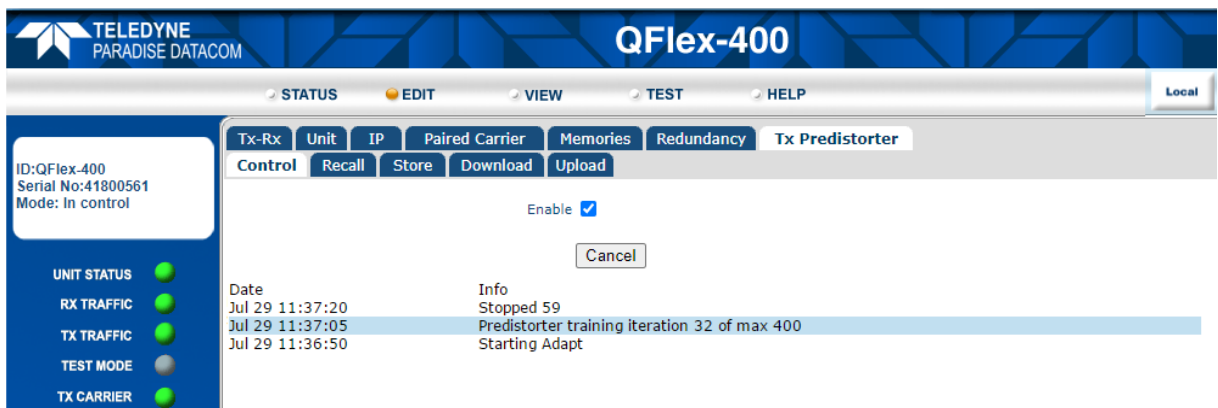
Figure 6-52 Edit->Tx Predistorter Screen (on completion of the learning process)
