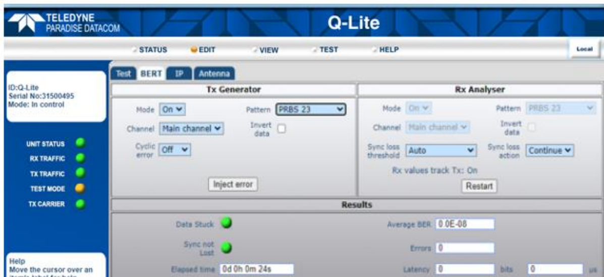
Figure 6-59 BER Test Generator/Analyser Screen
