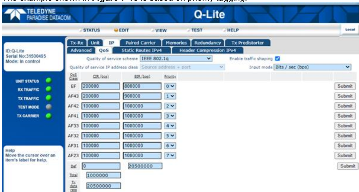
Figure 7-13 Traffic Shaping Configuration Screen using IEEE 802.1p Priority Tags
