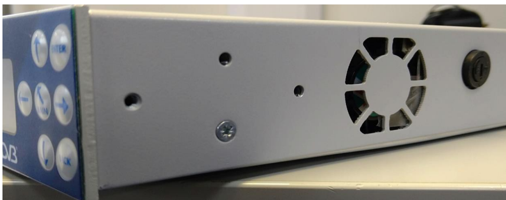
Figure 5-4A Q-Lite Halfwidth Fuse Location
