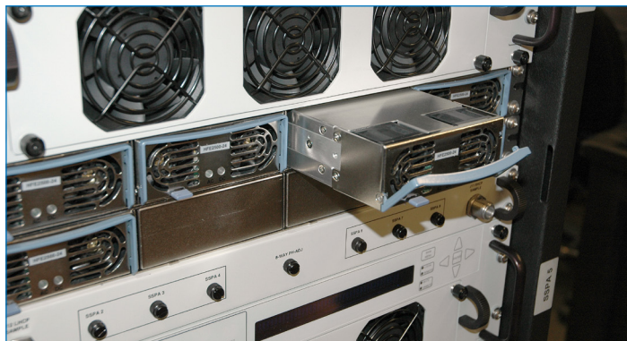
Power Supply Modules Removable from Front Panel
