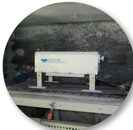
Conducted RF Immunity Signal applied: 150kHz-80 MHz, 10Vrms 1 kHz AM, 80% modulation
