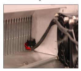
Figure 4: Unplug Fan Power (3RU Chassis shown)
