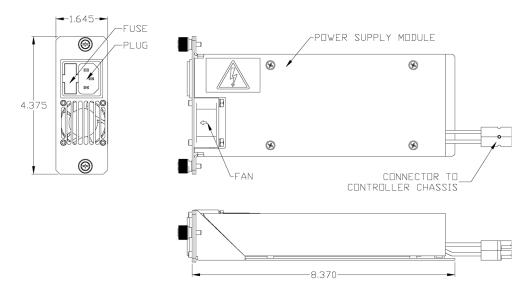
Figure 4: Outline Drawing, -HP Option Power Supply Module
