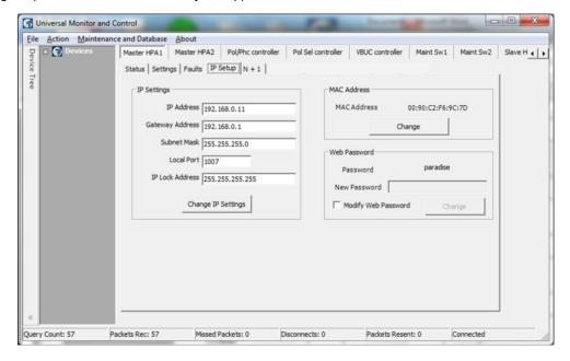
Figure 38: IP Setup Window, Outdoor SSPA Controllers
