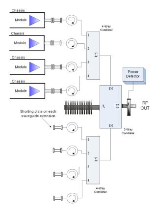
Figure 8: Eight-module PowerMAX System, Less 4 Modules
