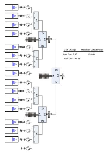
Figure 9: 16 Module PowerMAX Systems with 15 Modules
