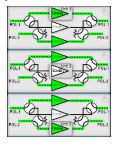
Figure 12: MIMIC Panels, with HPA2 on Standby in 1:2 System
