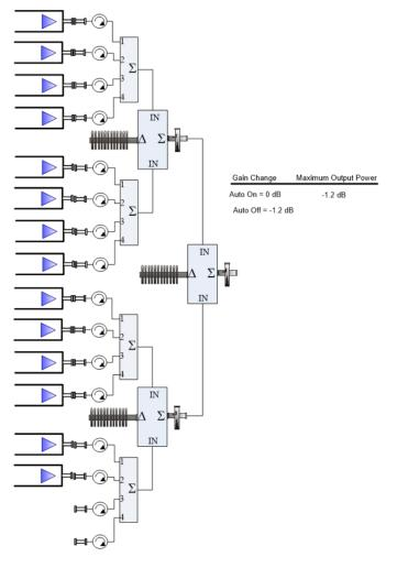
Figure 10: 16 Module PowerMAX Systems with 14 Modules
