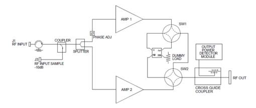
Figure 1: Block Diagram, 1:1 Phase Combined System
