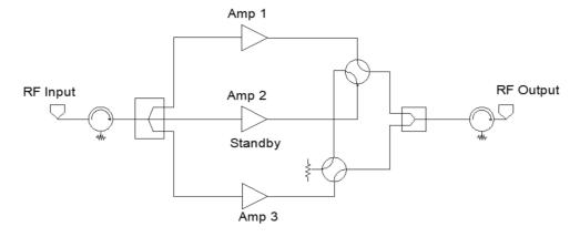
Figure 20: Block Diagram, 1:2 Fixed Phase Combined System
