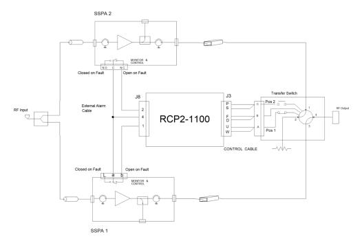
Figure 4: Schematic, Typical, 1:1 Redundant HPA System
