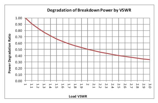
Figure 13: Degradation of Breakdown Power by VSWR
