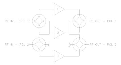
Figure 9: Block Diagram,1:2 Redundant System
