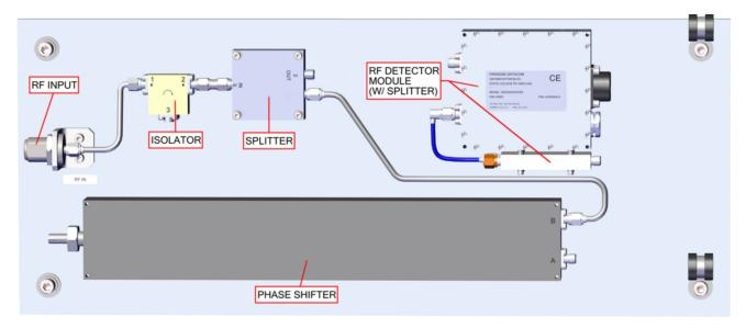
Figure 3: System Plate Assembly
