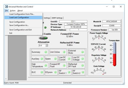
Figure 58: Universal M&C File > Load Last Configuration
