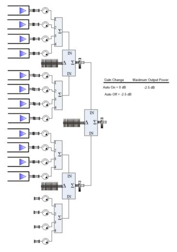
Figure 12: 16 Module PowerMAX Systems with 12 Modules
