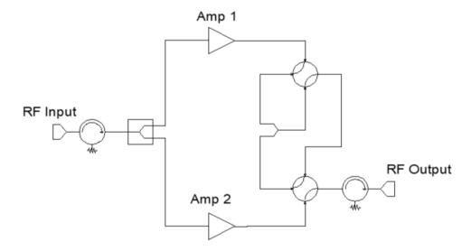
Figure 17: Block Diagram, 1:1 Fixed Phase Combined System
