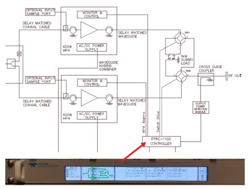
Figure 2: FPRC-1100 Phase Combined System Controller
