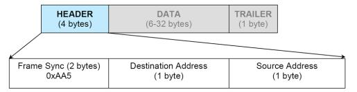
Figure 4: Header Sub-Packet
