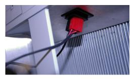
Figure 7: Unplug Fan Power (5RU Chassis shown)
