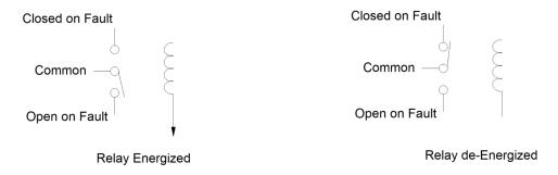
Figure 2: Parallel I/O Form C Relay
