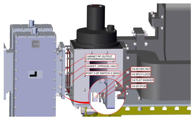
Figure 4: Connect Cabinet 2 (HPASS800AEZA002G2) to Switch Assembly
