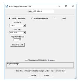
Figure 11: Add Compact Outdoor SSPA > Serial Connection
