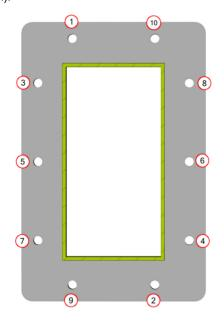
Figure 8: Torque Hardware in Star Pattern
