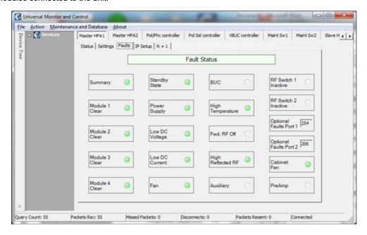
Figure 37: Faults Window, Outdoor SSPA Controllers
