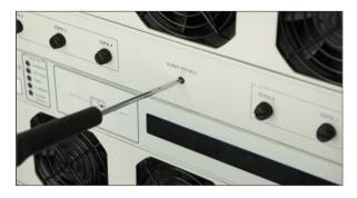
Figure 3: Adjust 8-Way Phase Trimmer
