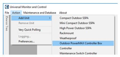
Figure 32: Universal M&C > Add Unit > Outdoor PowerMAX Controller Box
