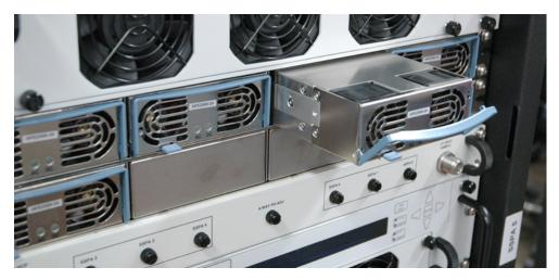
Figure 19: N+1 Power Supply with Removable Modules
