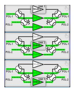
Figure 14: MIMIC Panels, with HPA1 on Standby in 1:2 System
