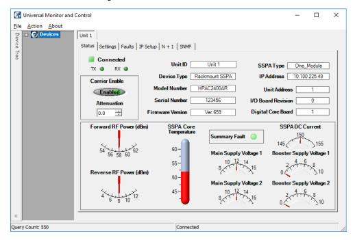
Figure 4: Universal M&C Software > Status Tab
