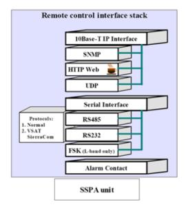
Figure 1: Remote Control Interface Stack
