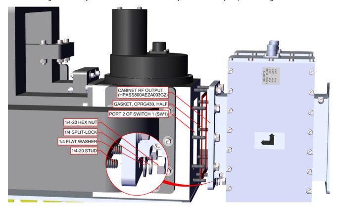
Figure 5: Connect Cabinet 1 (HPASS800AEZA003G2) to Switch Assembly
