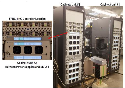
Figure 3: Location of FPRC-1100 Controller, Cabinet #2, Between Power Supplies and SSPA 1
