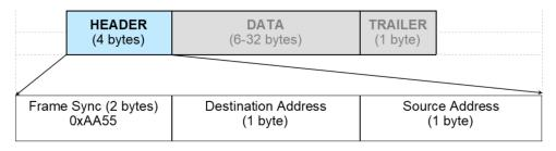
Figure 5: Header Sub-Packet
