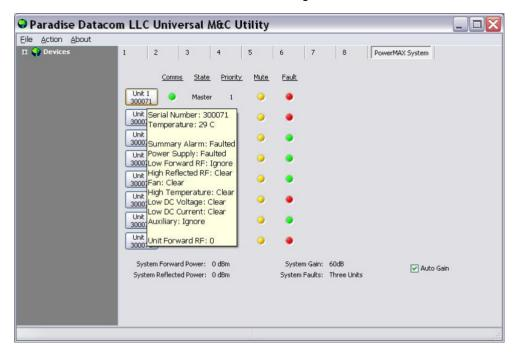
Figure 29: N+1 System Tab > Unit Info on Hover
