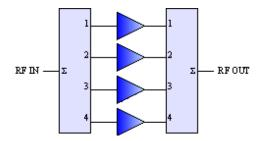
Figure 2: Block Diagram, Four-Module PowerMAX System
