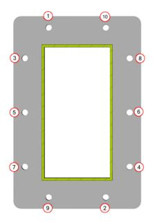
Figure 12: Torque Hardware in Star Pattern
