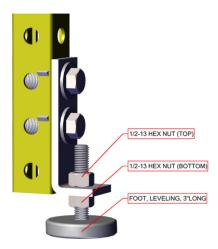
Figure 3: Detail, Leveling Foot
