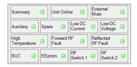
Figure 15: Status Tab > Fault Status Indicators
