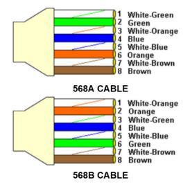
Figure 7: Wiring Using 568A and 568B Color Codes
