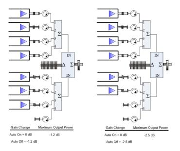
Figure 6: Eight Module PowerMAX Systems with 7 and 6 Modules
