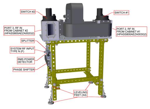
Figure 2: Switch Assembly
