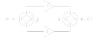
Figure 1: Block Diagram, 1:1 Redundant System
