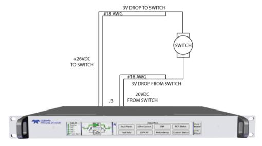
Figure 7: Cable Losses to Transfer Switch
