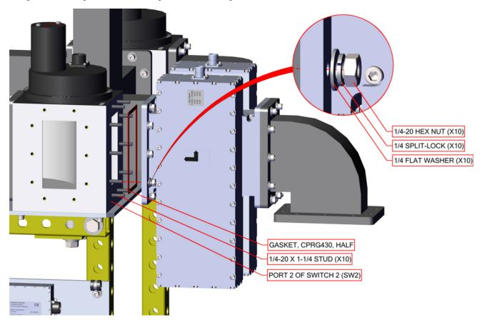
Figure 7: Install Crossguide Assembly
