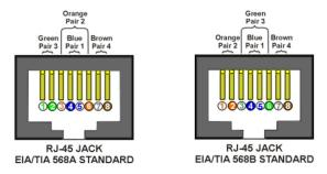
Figure 5: Ethernet Wire Color Code Standards
