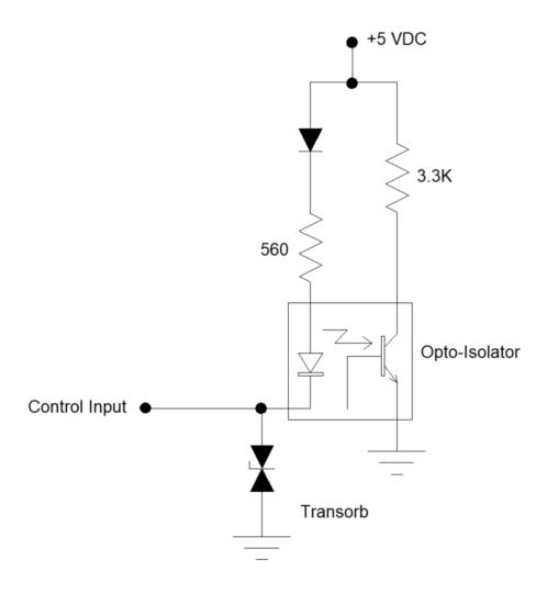
Figure 3: Opto-isolated Parallel I/O Input
