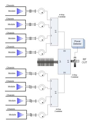
Figure 7: Eight-module PowerMAX System
