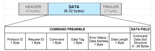
Figure 6: Data Sub-Packet
