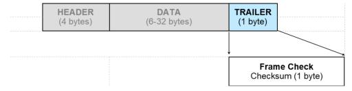
Figure 7: Trailer Sub-Packet
