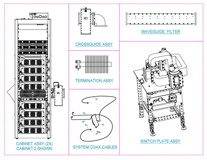
Figure 1: 1:1 FPC S-Band PowerMAX System Components, as Shipped
