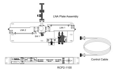
Figure 2: System Components, 1:1 Redundant System
