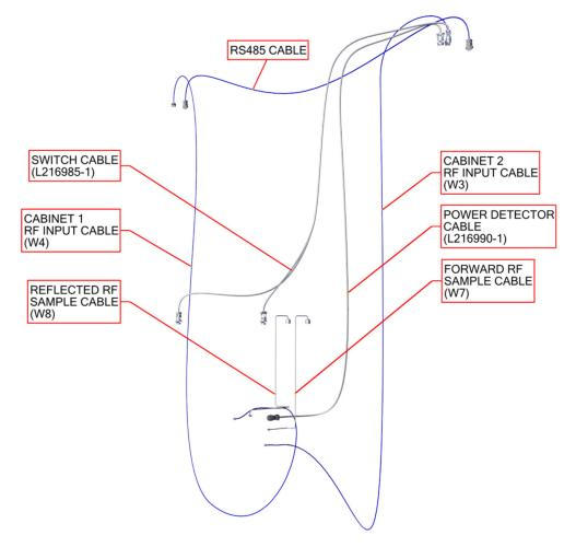
Figure 7: System Coaxial Cables
