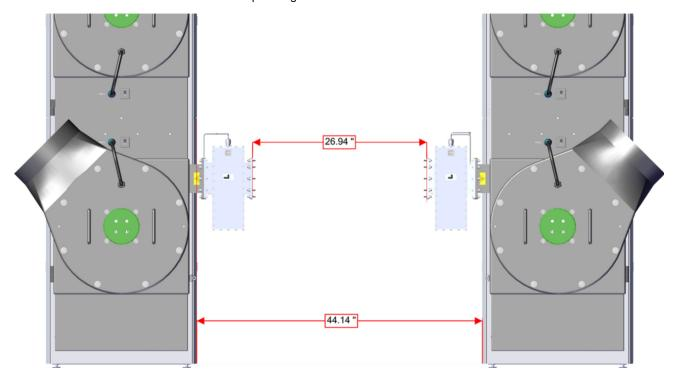
Figure 2: Dimensions, Space Between Cabinets and RF Output Flanges
