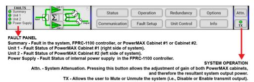
Figure 4: Fault Status and Action Buttons on FPRC-1100 Controller
