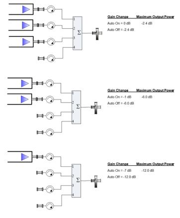
Figure 5: Four Module PowerMAX with 3, 2 and 1 Modules
