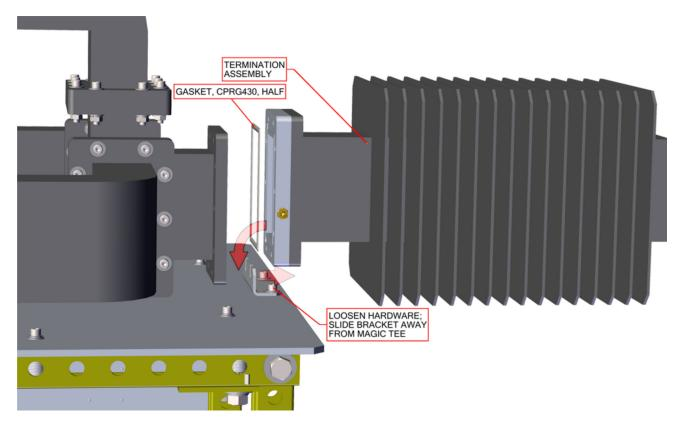
Figure 10: Slide Bracket, Install Gasket
