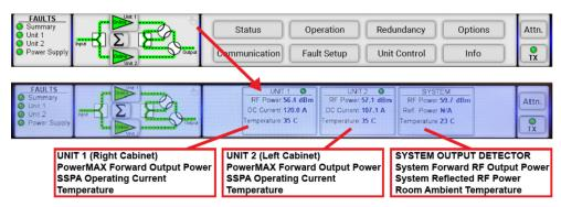
Figure 5: Monitor Status of Cabinets and System from RCP
