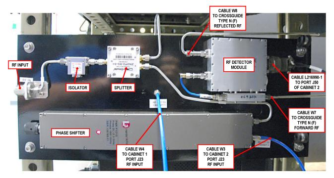
Figure 14: Connections to System Plate Assembly
