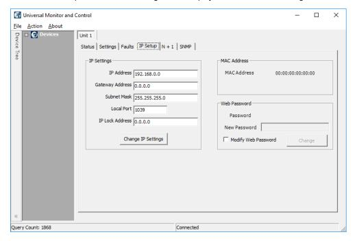
Figure 7: Universal M&C Software > IP Setup Tab
