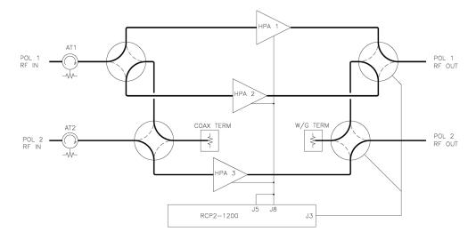
Figure 12: Block Diagram, SSPA 1:2 Redundant System
