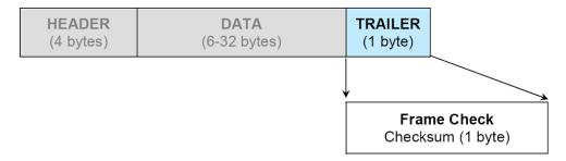
Figure 6: Trailer Sub-Packet
