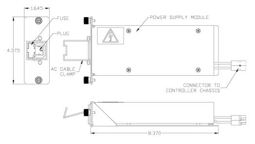
Figure 3: Outline Drawing, 24V Power Supply Module
