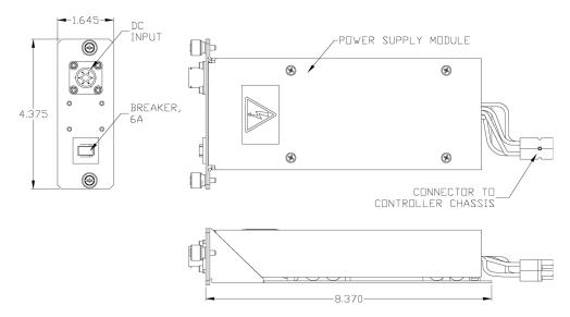
Figure 5: Outline Drawing, 48V Power Supply Module
