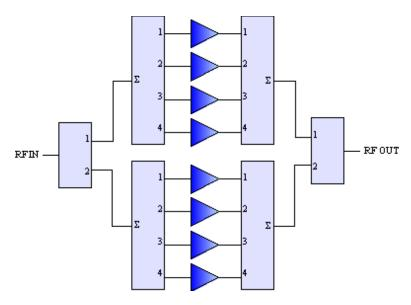
Figure 3: Block Diagram, Eight-Module PowerMAX System
