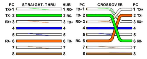
Figure 6: Wiring Using 568A Color Codes
