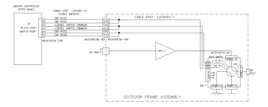
Figure 26: Schematic, SSPA Utilizing Maintenance Switch and Controller
