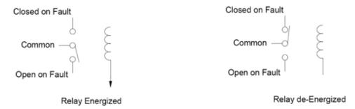
Figure 2: Parallel I/O Form-C Relay
