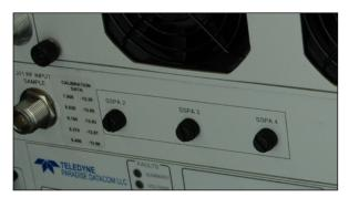
Figure 2: Phase Adjusters for SSPA 2, SSPA 3 and SSPA 4
