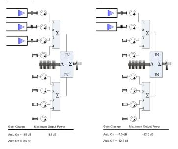
Figure 8: Eight Module PowerMAX Systems with 3 and 2 Modules
