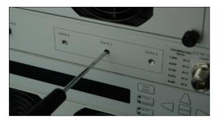
Figure 4: Adjusting Phase of SSPA 6, SSPA 7 and SSPA 8
