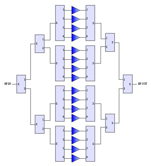
Figure 4: Block Diagram, 16-Module PowerMAX System
