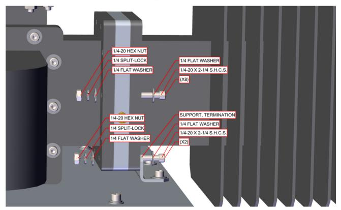
Figure 11: Bolt W/G Flanges Together
