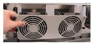
Figure 6: Remove Front Fan Assembly (5RU Chassis shown)
