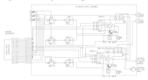
Figure 11: Schematic, Typical, 1:2 Redundant LNA System
