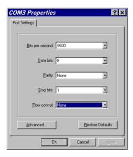
Figure 10: HyperTerminal Communication Properties
