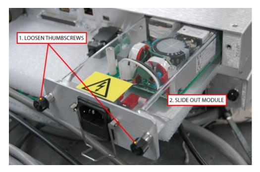
Figure 5: Loosen Thumbscrews and Slide Module from Chassis
