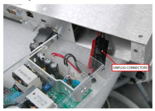
**Figure 6: Unplug Power Pole Connectors**
