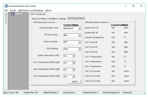
Figure 45: Universal M&C, HPA Control Panel Window
