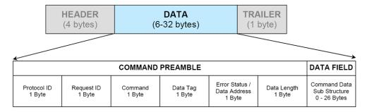
Figure 5: Data Sub-Packet
