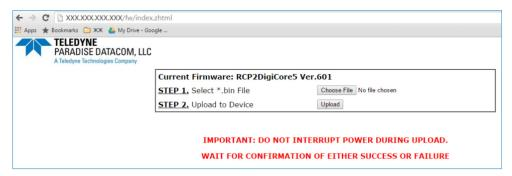
Figure 8: Firmware Upgrade, Upload code.bin File
