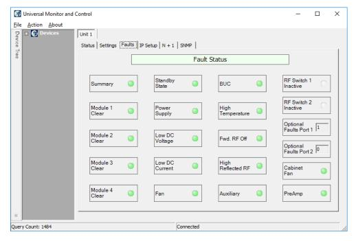
Figure 6: Universal M&C Software > Faults Tab
