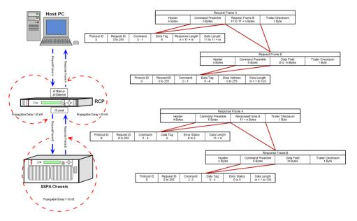
Figure 7: Packet Wrapper Technique
