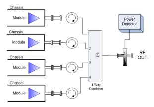
Figure 6: Block Diagram, Four-way PowerMAX System
