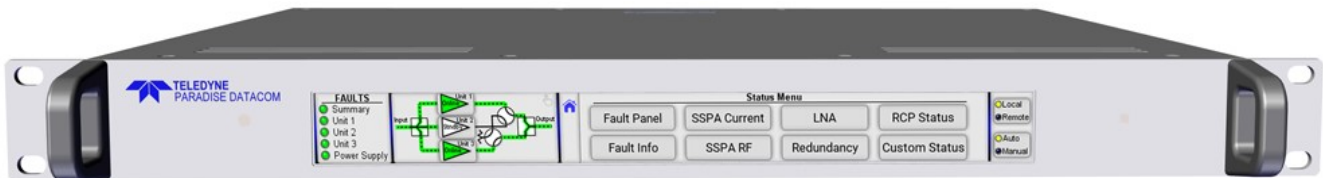
CONTROLLER CONFIGURED FOR 1:2 PHASE COMBINED SYSTEM
