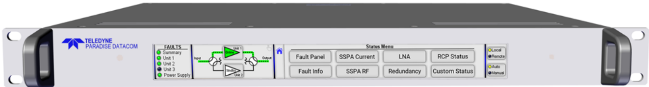
CONTROLLER CONFIGURED FOR 1:1 REDUNDANT SYSTEM
