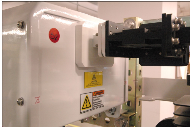
Figure 2-8: Secure RF Output Flange to Waveguide Assembly
