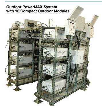
**Teledyne Paradise Datacom's** Outdoor PowerMAX system is a purely parallel redundant, modular HPA system. It can be populated with four, eight, or sixteen modules. The Outdoor PowerMAX system with either use the popular Compact Outdoor SSPA module, or the High Power Outdoor module.
