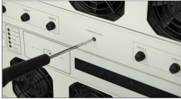
Figure 3: Adjust 8-Way Phase Trimmer
