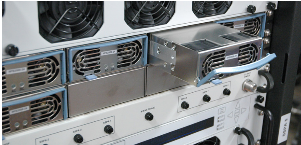
Figure 19: N+1 Power Supply with Removable Modules
