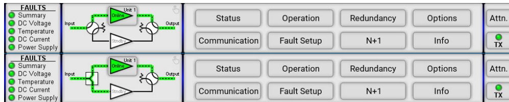
Figure 71: Mimic Panels Showing Input Switching (top) and Input Splitting (bottom)
