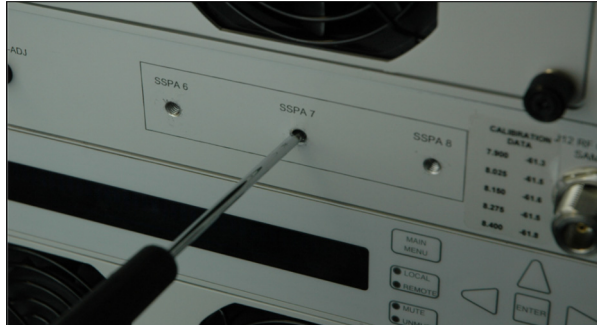
Figure 4: Adjusting Phase of SSPA 6, SSPA 7 and SSPA 8
