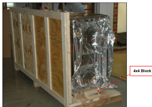
Figure 3: Remove Crate Side Walls
