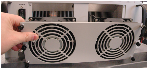
Figure 6: Remove Front Fan Assembly (5RU Chassis shown)
