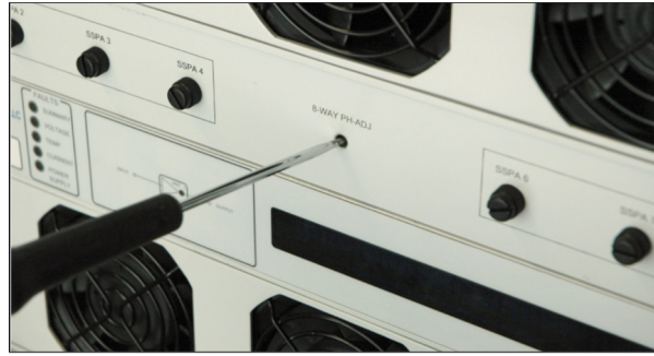
Figure 5: Adjust 8-Way Phase Trimmer
