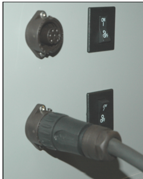
Figure 13: Connect Power Cables to Impeller
