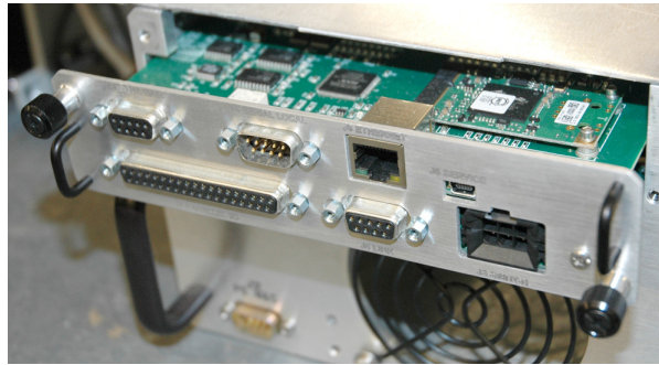
Figure 11: Slide Card from Chassis to Access Programming Connectors
