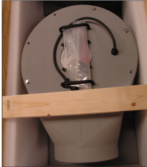
Figure 14: Exhaust Impeller, as Shipped
