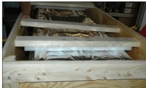
Figure 2: Remove and Save Shipping Brackets
