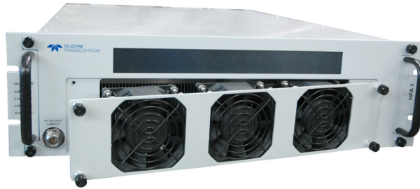
Figure 3: Remove Front Fan Assembly (3RU Chassis shown)
