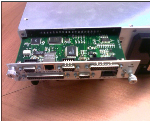
Removable rear panel monitor and control card
