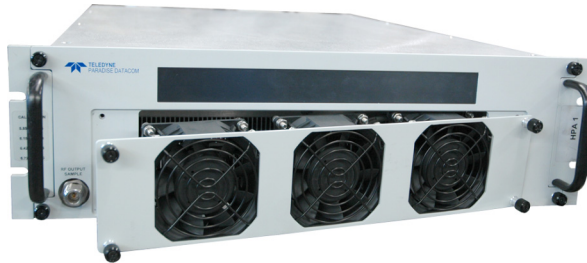
Figure 3: Remove Front Fan Assembly (3RU Chassis shown)
