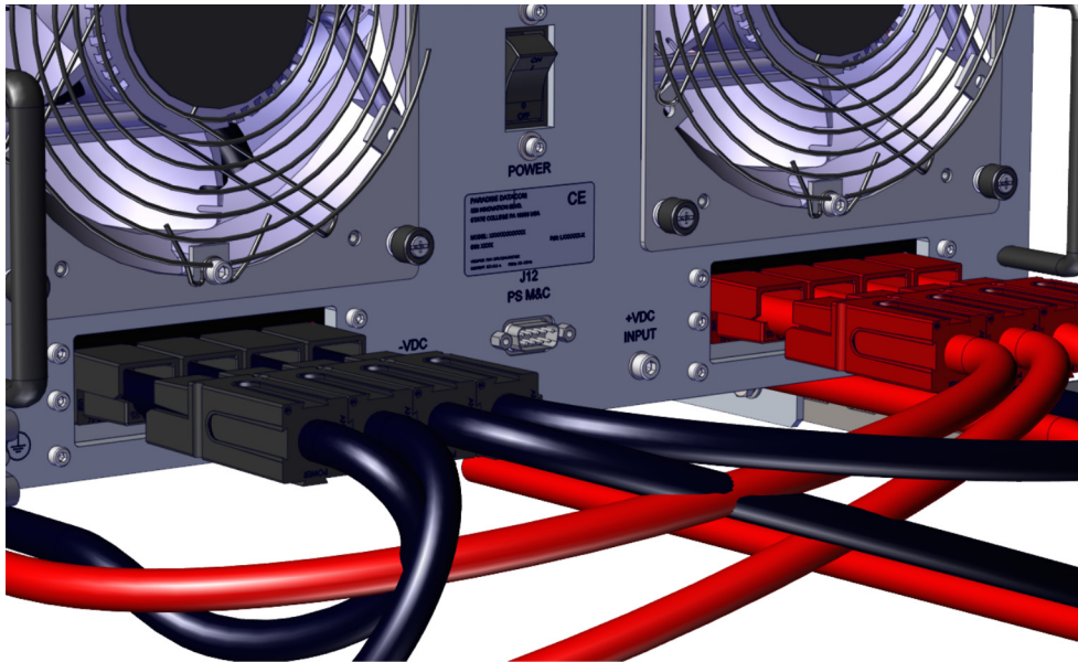
Figure 2: Connect DC Cable Power Pole Connectors (7RU shown)
