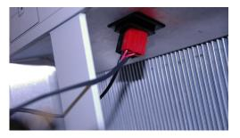
Figure 7: Unplug Fan Power (5RU Chassis shown)
