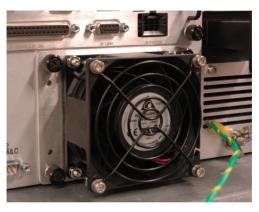
Figure 8: Unscrew Thumbscrews to Remove Rear Fan Assembly (3RU Chassis shown)
