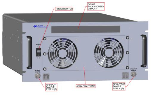
Figure 1: 5RU SSPA, Front Panel
