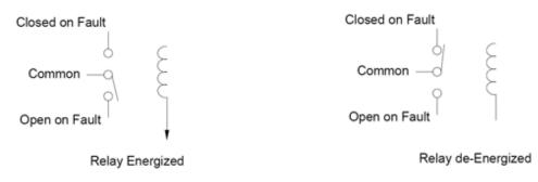
Figure 2: Parallel I/O Form-C Relay
