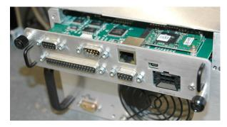
Figure 11: Slide Card from Chassis to Access Programming Connectors
