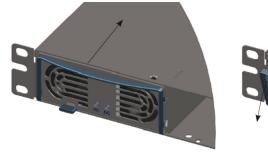
To insert the power supply push unit into the rack with extraction handle closed.
