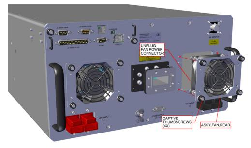
Figure 4: 5RU SSPA, Rear Fan Assemblies
