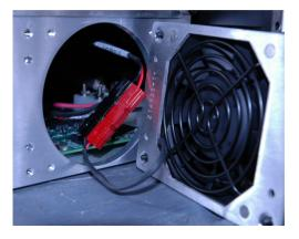
Figure 9: Unplug Fan Power (3RU Chassis shown)
