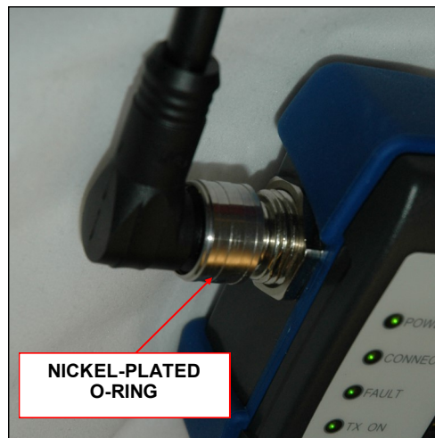
Figure 2-4: Pull on O-Ring to Remove Cable from Controller
