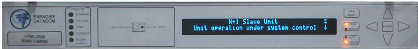
Figure 3-11: Front Panel Display, Slave Unit (Online LED Dark)
