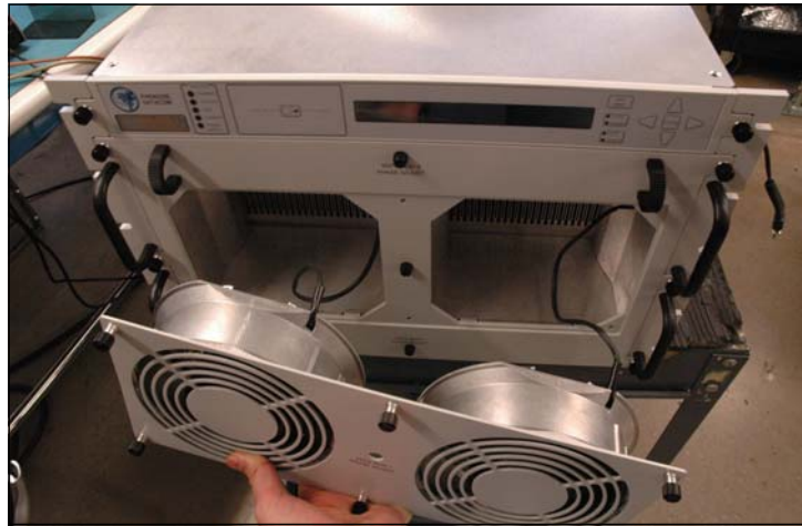
Figure 4-12: Remove Front Panel Fan Tray
