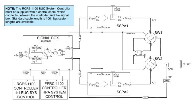
The Block Up Converter system is housed in a weather-proof enclosure (shown below) and is controlled by an indoor RCP2-1100 Redundant Controller. The Teledyne Paradise Datacom ZBUC<sup>®</sup> converter architecture allows a converter that is fitted with an internal reference oscillator to automatically detect and switch to an externally applied 10 MHz reference signal.
