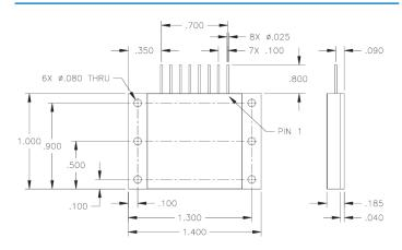
Drawing shows the hermetic package, mounting flange and 8 external connections. All dimensions given are inches, tolerances  $\pm 0.005$ . The package walls are 0.040 inch thick, cover is 0.010 inch thick. Pin 1 is top-right in the diagram.
