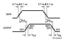
FIGURE 3. Propagation and Transition Times
