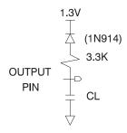
Note: CL = 100 pF including jig capacitance except -55 devices, where CL = 30 pF.
