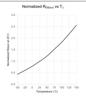
Figure 12: Normalized  $R_{\text{DS(on)}}$  as a function of  $T_{\text{J}}$
