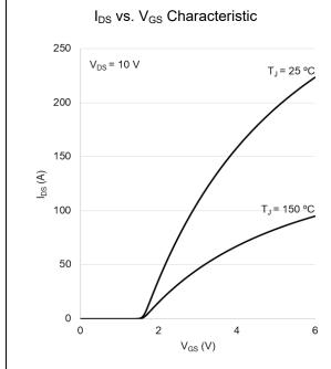
Figure 11: Typical I<sub>DS</sub> vs. V<sub>GS</sub>
