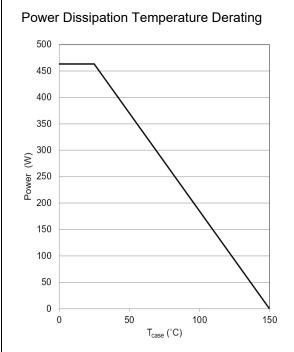
Figure 17: Derating vs. Case Temperature
