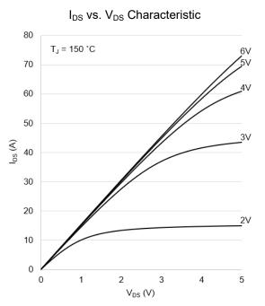
Figure 2: Typical I<sub>DS</sub> vs. V<sub>DS</sub> @ T<sub>J</sub> = 150 °C
