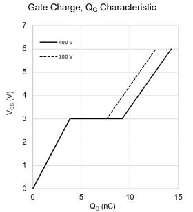
Figure 6: Typical VGS vs. QG @ VDS = 100, 400 V
