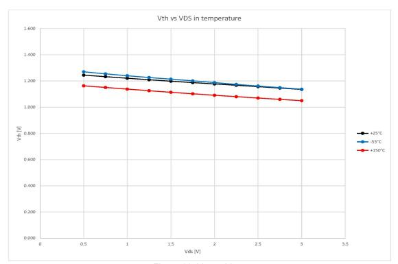
Figure 18: V<sub>TH</sub> vs V<sub>DS</sub>
