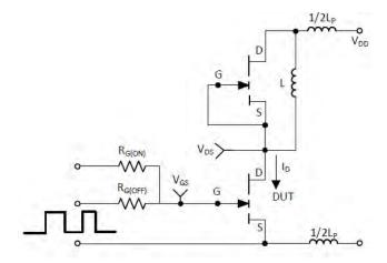
Figure 23: Switching Loss Test Circuit
