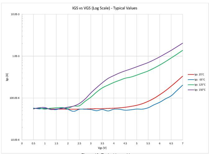
Figure 13: Typical I<sub>GS</sub> vs V<sub>GS</sub>
