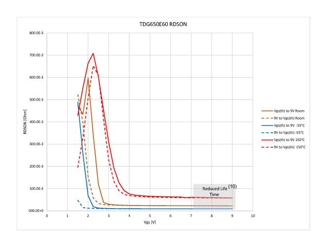
Figure 20:  $R_{DS(ON)}$  vs  $V_{GS}$  vs Temp
