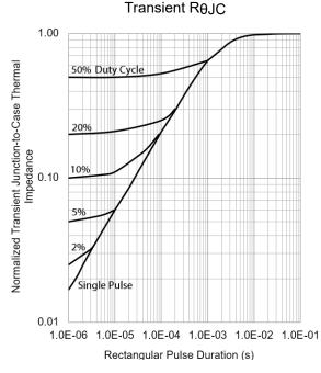
Figure 16: Transient Thermal Impedance (1.00 = Nominal dc thermal impedance)
