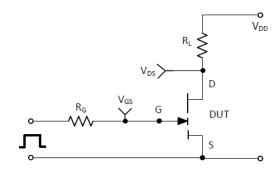
Figure 21: switching time test circuit
