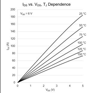
Figure 5: Typical IDS vs. VDS @ VGS = 6 V
