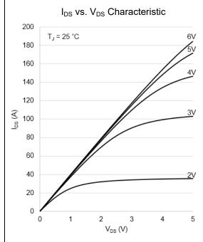
Figure 1: Typical I<sub>DS</sub> vs. V<sub>DS</sub> @ T<sub>J</sub> = 25 °C
