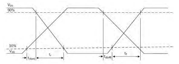
Figure 22: switching time waveforms
