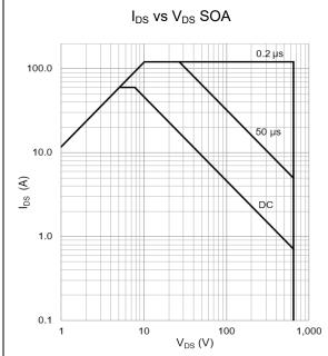
Figure 14: Safe Operating Area, T<sub>case</sub> = 25 °C
