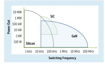
Many industries have their equivalent of the Moore's Law graph, an illustration that neatly encapsulates the hopes of a market and is published repeatedly. For this segment, it is shown above, and displays the approximate switching speed of available devices against the achievable power levels for different technologies.
