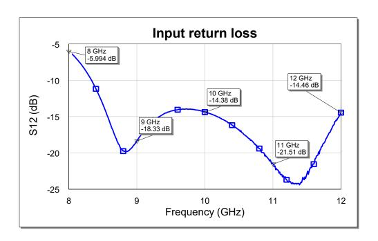
Test fixture data for Bare Die Vd1 = Vd2 = 2 V, Vd3 = 5 V, Total Current = 80 ma, T<sub>A</sub> = 25 °C
