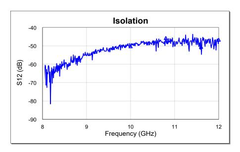
Test fixture data for Bare Die Vd1 = Vd2 = 2 V, Vd3 = 5 V, Frequency = 9.6 GHz Total Current =75 ma, Тд = 25 °C
