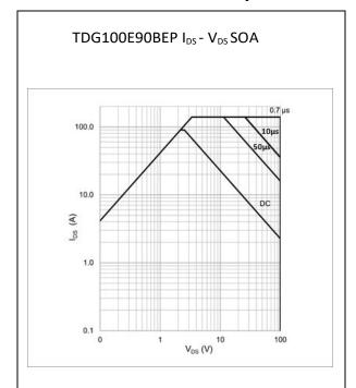
Figure 16: Safe Operating Area @ T<sub>case</sub> = 25 °C
