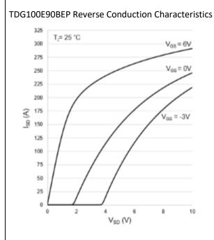
Figure 9: Typical I<sub>SD</sub> vs. V<sub>SD</sub> at T<sub>J</sub> = 25°C
