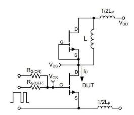
Figure 20: TDG100E90BEP Switching Loss Test Circuit
