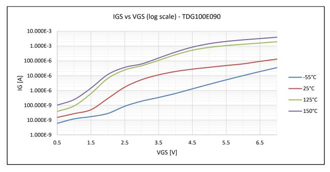
Figure 14: IG vs VGS (log scale) - Typical Values
