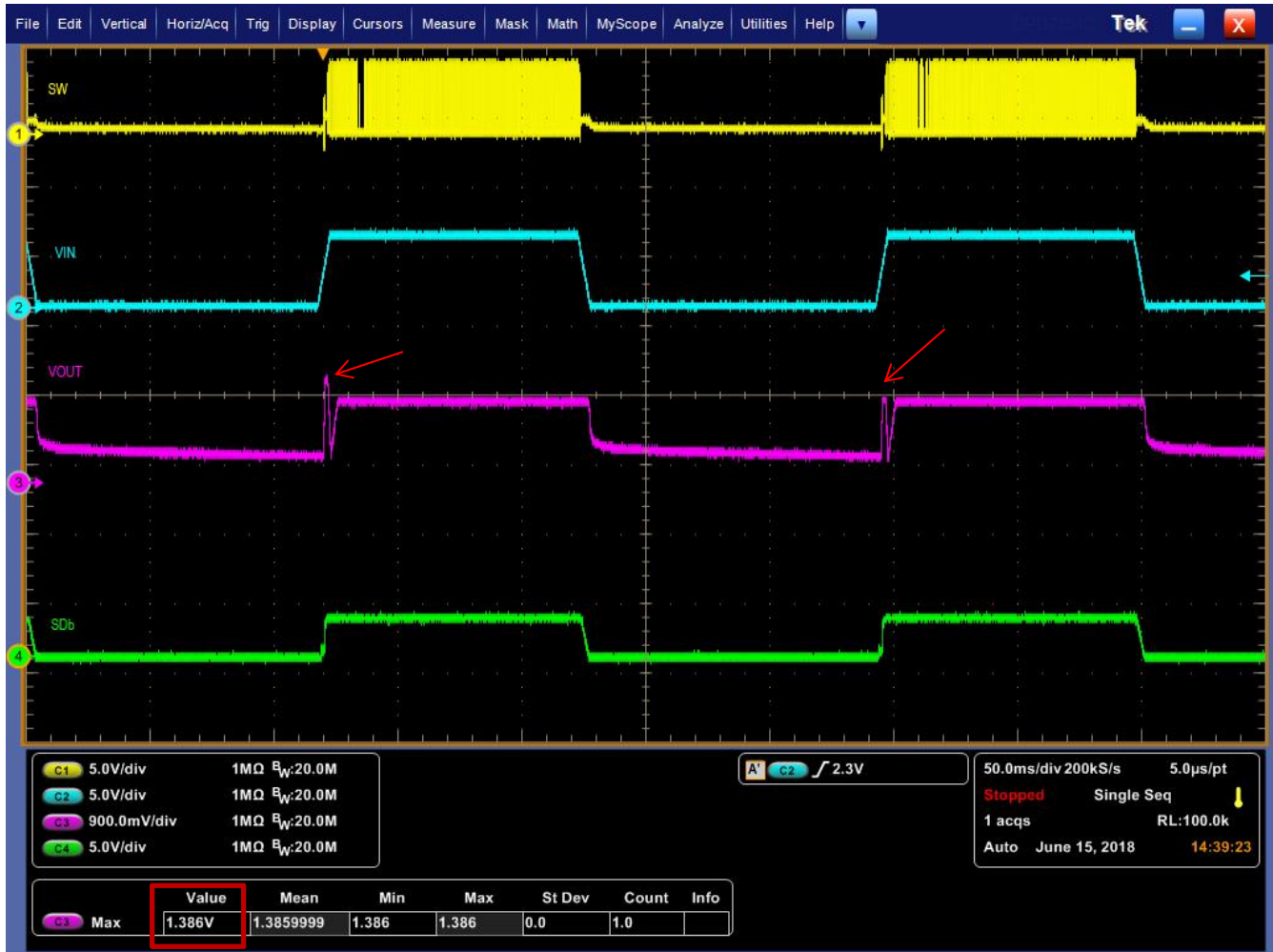
Figure 4. Plot of Same Unit, with the VIN Slew Rate Reduced to 1,000 V/s
