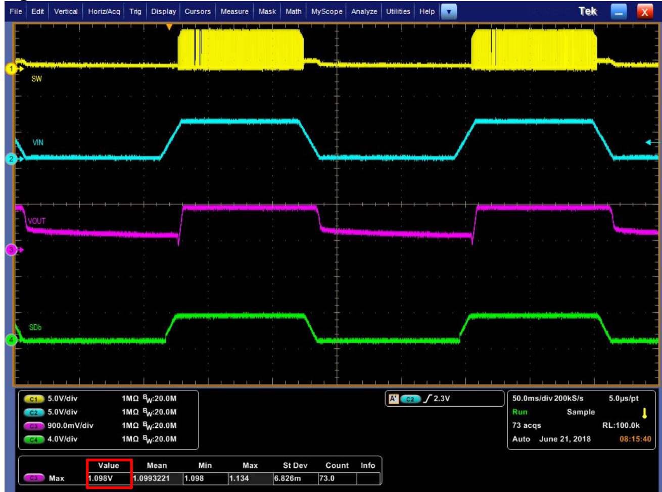
Figure 6. Plot of Sam Unit, with VIN Slew Rate Reduced to 300 V/s.
