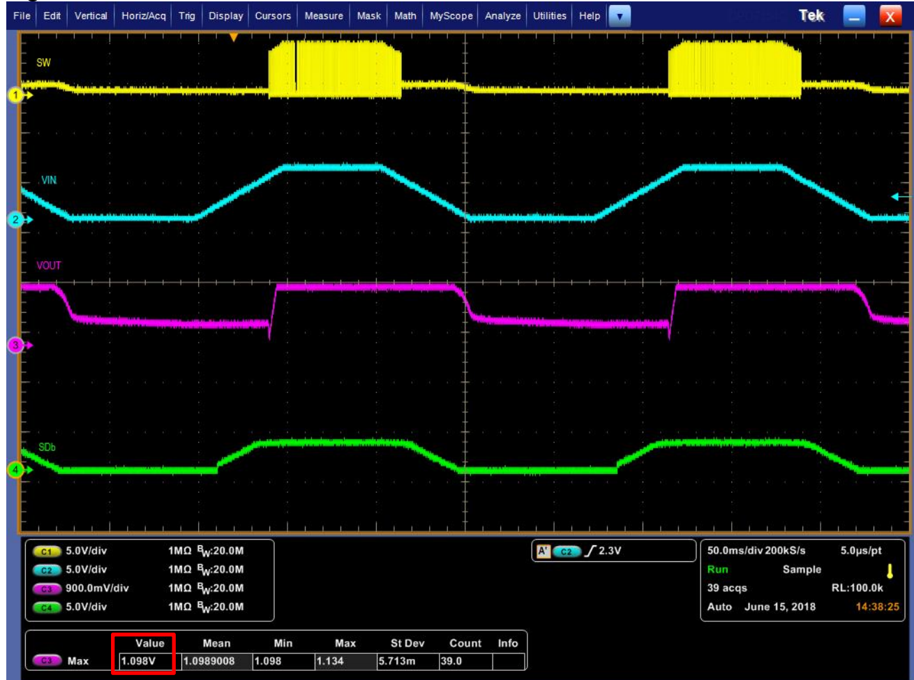
Figure 7. Plot of Sam Unit, with VIN Slew Rate Now Reduced to 100 V/s.
