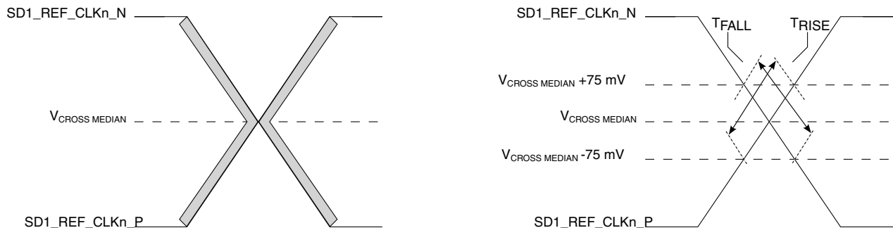
Figure 3-62. Single-ended measurement points for rise and fall time matching
