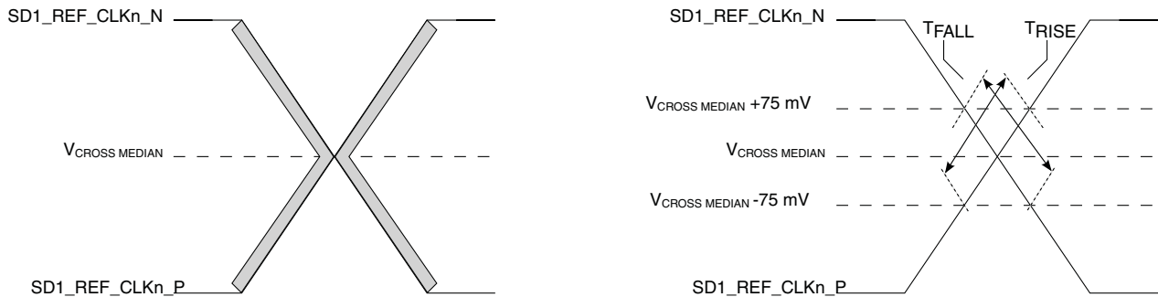
Figure 3-63. Single-ended measurement points for rise and fall time matching
