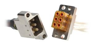
A smaller, multi-pin version of the PeeWee series of high voltage connectors and cable assemblies. Although micro-miniature in size, this series of cable assemblies will operate at voltages up to 6 kVDC at 70,000 ft (21.34 km) altitude over a temperature range of -55° to 125° C.
