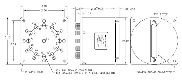
\*D-Sub with Indicator Contacts= 2.26 MAX \*D-Sub with additional option = 3.20 MAX
