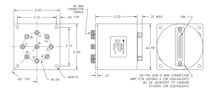
"-S Option" 25-Pin D-Micro Connector (Example: CCR-58S180-S)
