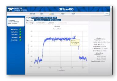
**Spectral view:** The Rx Spectrum Monitor is a powerful real-time spectrum analyser within the modem that is used to view the received signal spectrum. The monitor can not only display the wanted carrier but a Super Wide view allows checking for adjacent interfering carriers.
