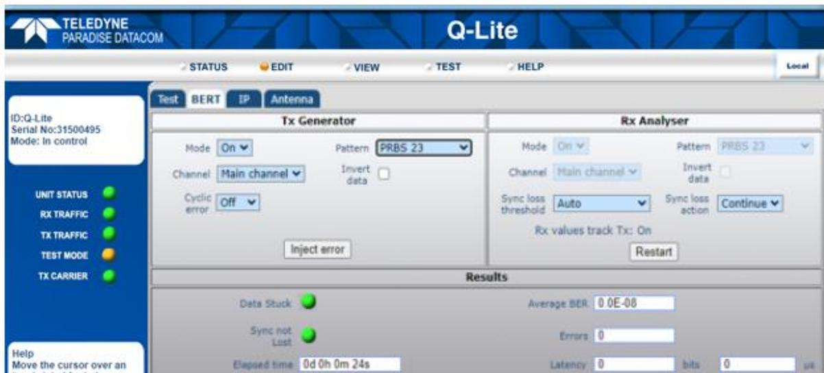
**Figure 6-59 BER Test Generator/Analyser Screen**
