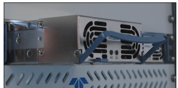
Power Supply Module in Chassis
