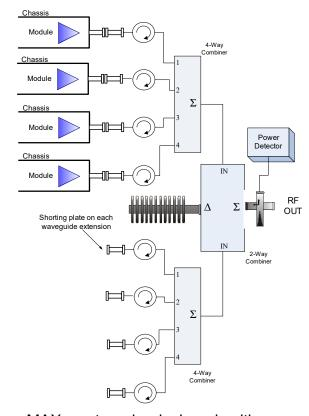
number of active modules vary. The Outdoor PowerMAX system is designed with an Auto-Gain Control mode so that the overall system gain will remain constant in the event of a single module failure. See the table below.
