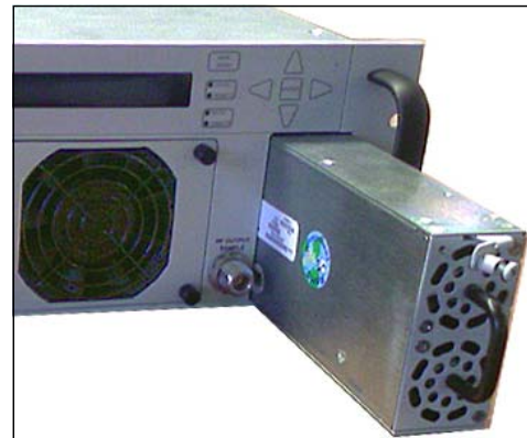
Figure 3-9: Remove Power Supply Module
