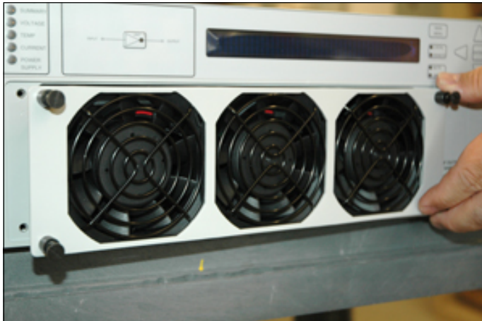
Figure 3-2: Unscrew Thumb Screws on Fan Tray and Slide Tray from Chassis
