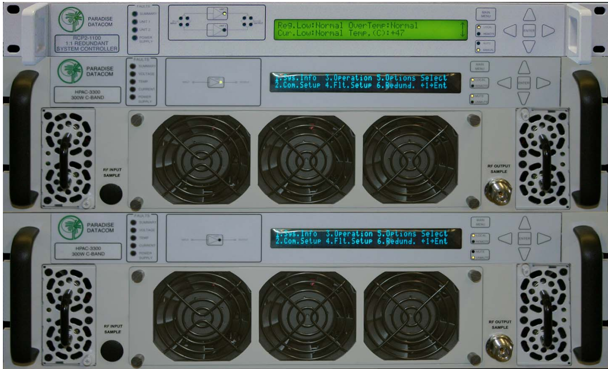
Figure 4-2: RM SSPA 1:1 Redundant Systems
