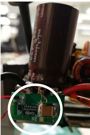
PFC with transition-mode controller L6562A (Side View)
