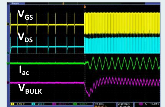
Full load to no load (0.5A to 0A)
